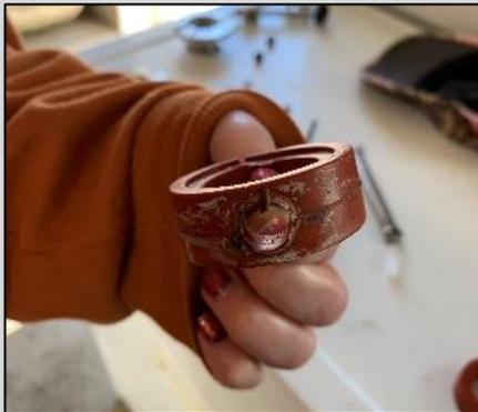
Pictured above is a valve from a pasteurizer that was causing high bacterial counts in the milk fed to the calves.
