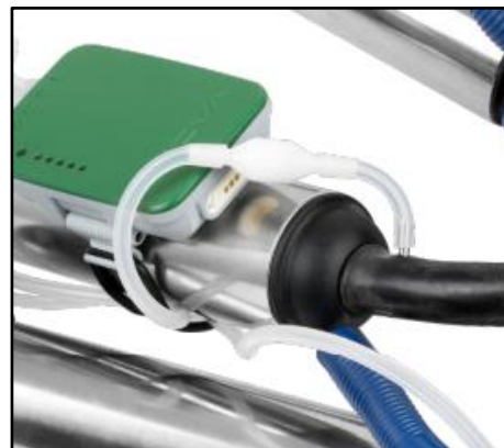
The VaDia is pictured above in blue strapped to the teat cup of a milking unit and at left it is in a green case. It collects vacuum readings.
